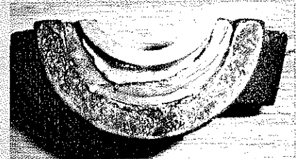
Above: The main bearings in both the block and the caps have been rebabbitted in an odd manner, with the babbitt apparently poured around a replaceable bearing insert, thus partially melting the insert. One main bearing cap stud bolt was in upside down.
